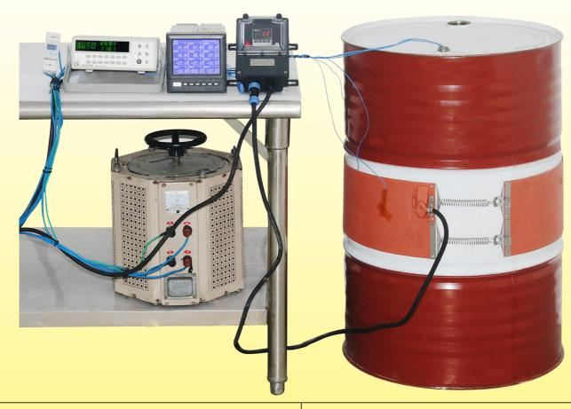
Variation in the temperature versus time of a 220-liter metal drum, filled with water, heated by a silicone heating belt 200mm wide, without thermal insulation, power 1500W (surface load 0.5W/cm²).
